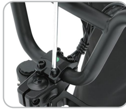
11. Tighten the four bolts on the headset retainer with a tool
