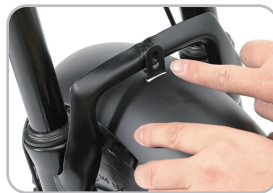
2. Align the fender mounting holes with the fork brace holes
