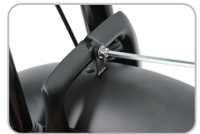
3. Tighten the screws to secure the fender to the fork brace
