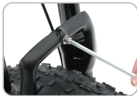
1. Remove the center screw from the fork brace
