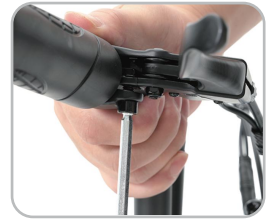
12. Tighten the screws on both brake levers to secure them
