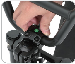
10. Install the headset retainer clip
