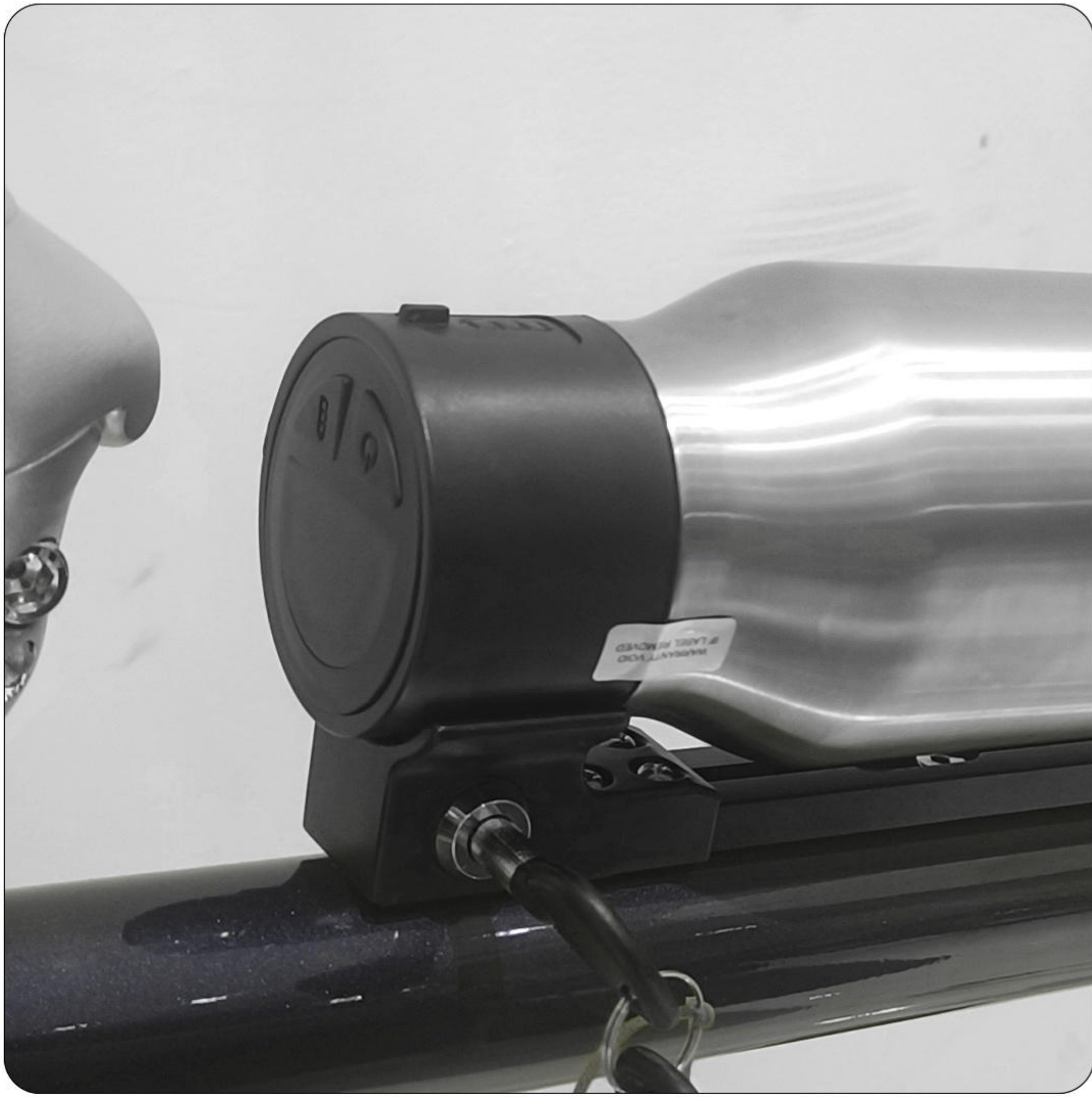
1. Turn key to unlock battery.
