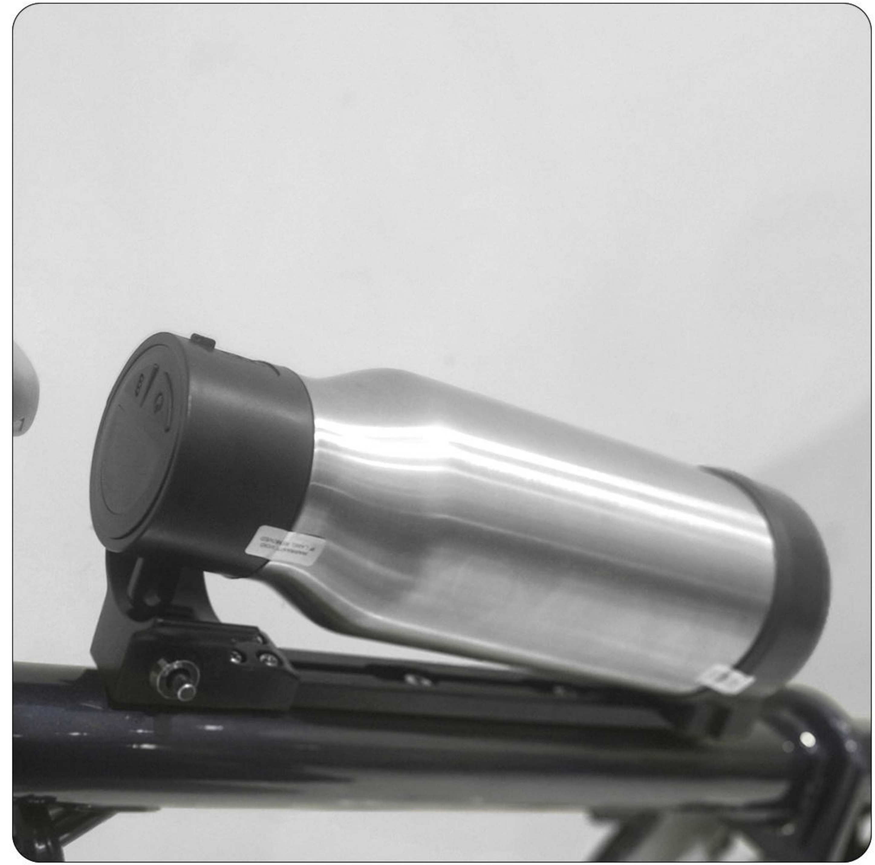
2. Pick up the battery upwards.
