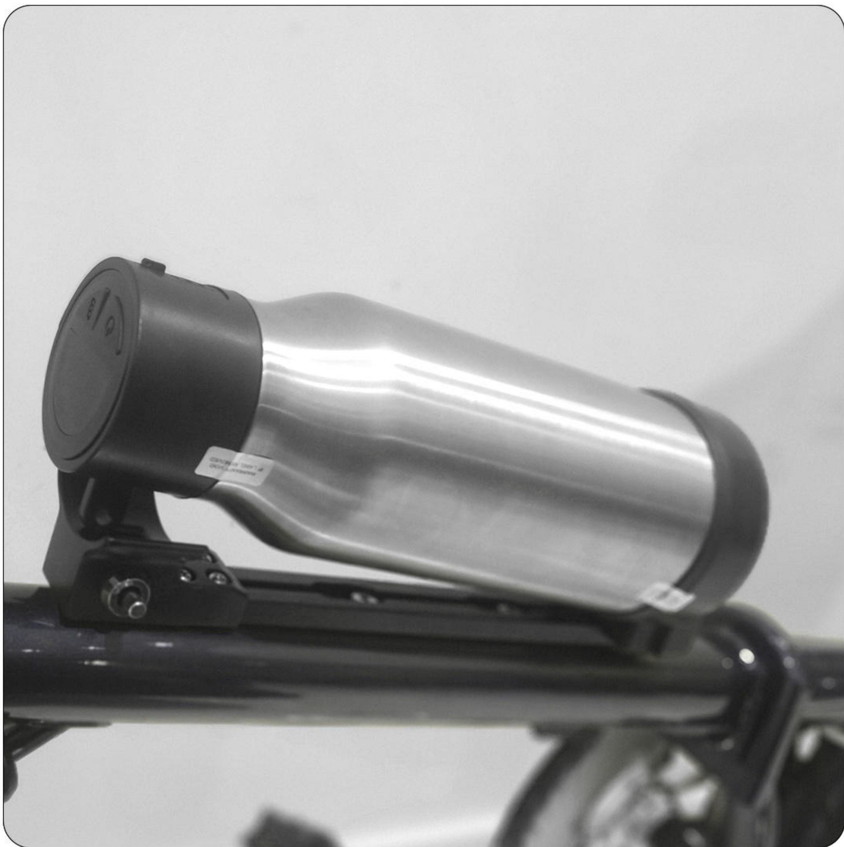
1. Install the battery, noting the connector underneath the battery.
