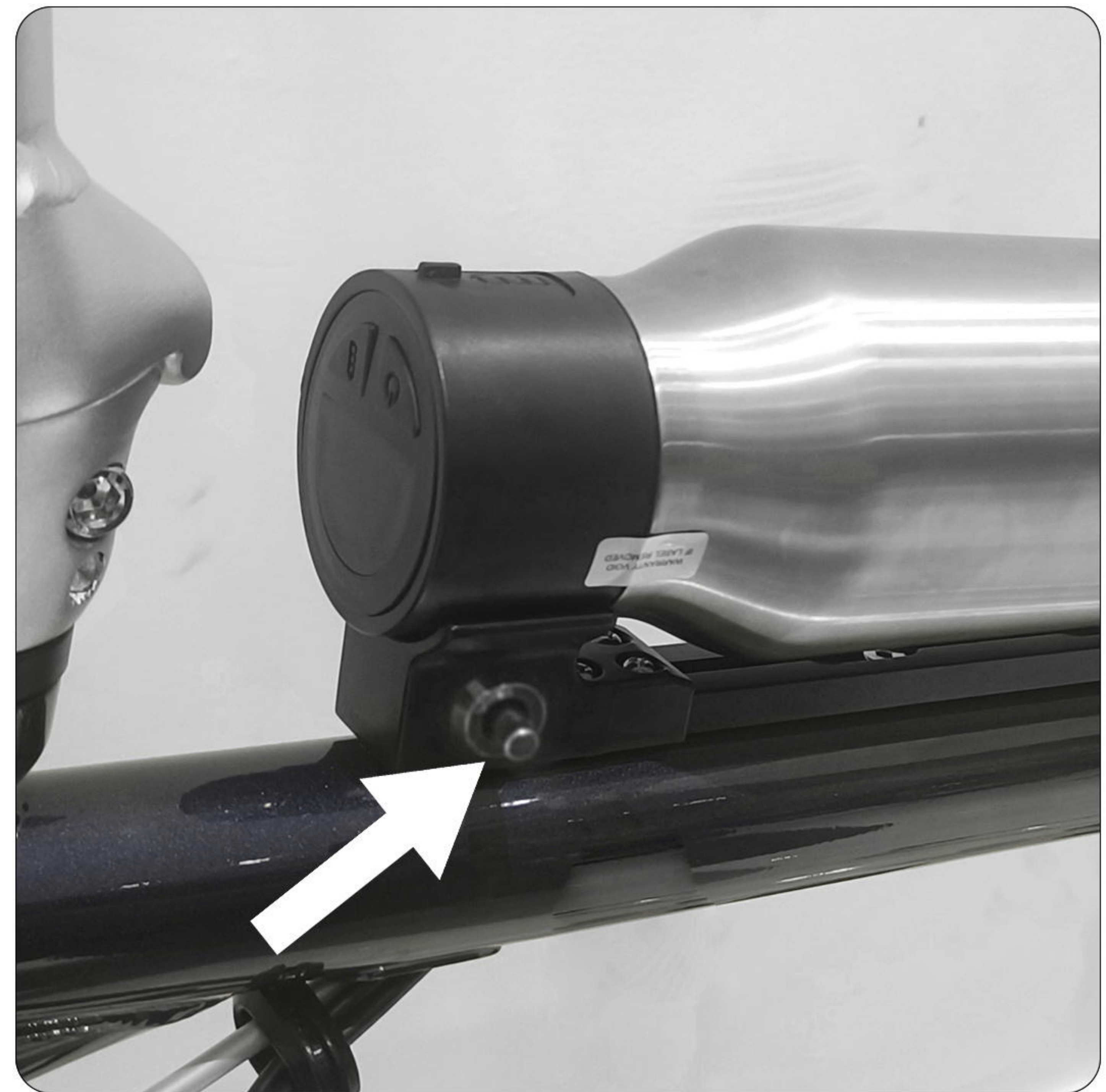
2. Press the latch on top of the battery lock.
