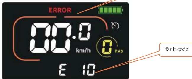
Caption: Error: ERROR flag, E10 indicates the error code
