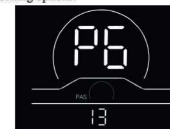
Fig. 4-6 Current Limit Setting Interface
