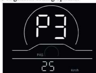
Fig. 4-3 Speed Limit Setting Interface
